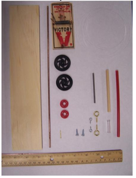
Mouse trap (1) Rear wheels inserts (2) Used CDs (2) Front wheels (2) Wooden board (1) Fishing line Large eyelet (2) Wooden dowel – rear axle (1) Small eyelet (2) Small nail (1) Short metal rod – front axle (1)Long metal rod – lever Wood screws (2) Clear plastic tube
