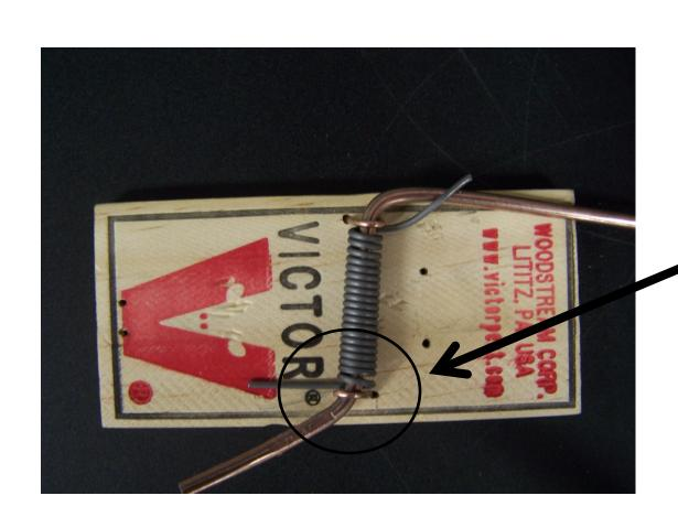
Bend the other end of the rod to secure the rod from sliding out.
